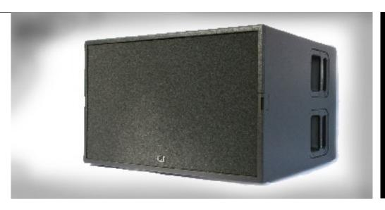
Concept: Ultra compact light wieght high output two chamber bandpass design with bass reflex tuning and two impulscompensated 15 inch chassis. Extreme stiff housing either flown or ground stacked. The big brother of the "die1B", the "die2B" offers more power and extended frequency response.
